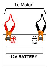
One battery gives 30 A-H with 30 Amp Drain over 1 Hr will go 4 mi at 4mph.
